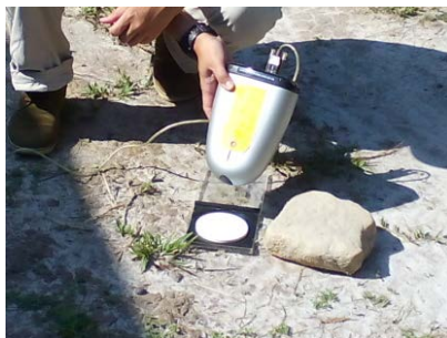
Figure 4: Reflectance's test in site SBIA- an ancient jetty structure (ancient brick) dated early of the 2 nd century CE using Spectroradiometer
