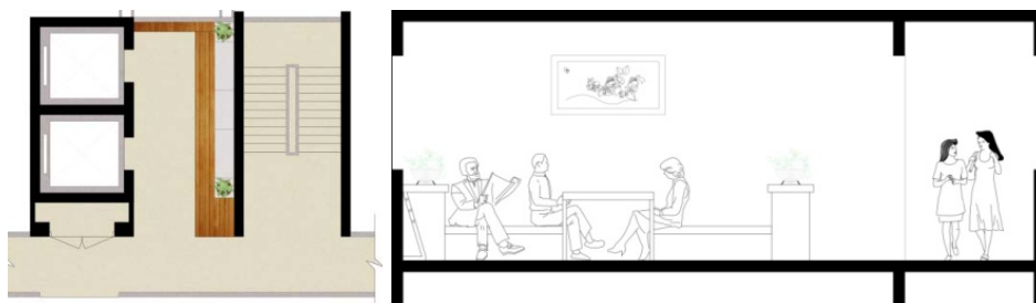
Figure 15 & 16: Redesigned lift lobby with a narrow width by adding built-in furniture and demarcated zones with differentiated materials, using the lift lobby layout from Figure 6.
