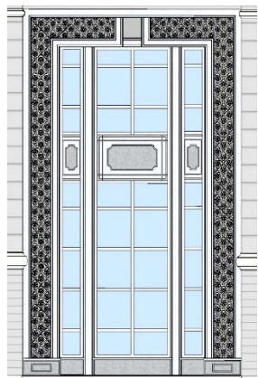
Figure 21: Window and door decorated with GFRG of hibiscus patterns. Sources: Kumpulan Senireka Sdn. Bhd, 2017
