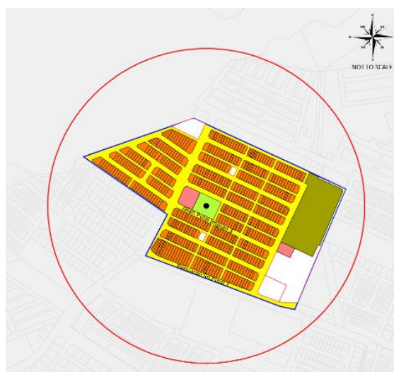
Figure 4: Taman Pulau Impian, Seremban. The residential area has only 1.271ha of open space but it covers the whole 400m radius of the residential units
