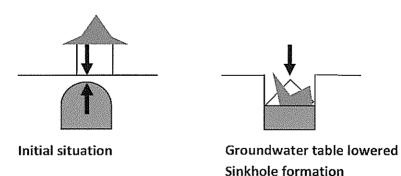
Figure 2: Simplified illustration of sinkhole formation mechanism.
