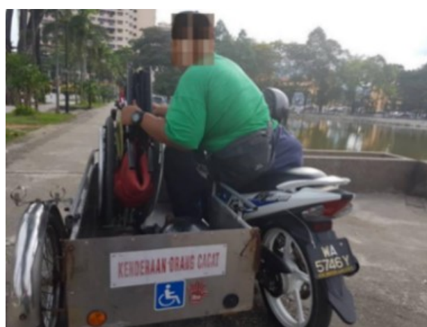
Figure 4: Motorcycle with wheelchair compartment Source: Kamarudin (2021)
