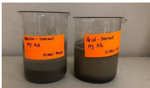
Figure 1: Fly ash soaked in HCl and NaOH
