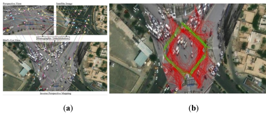
Figure 5: Inverse perspective mapping. (a) Overlaying video footage on satellite image, (b) Transforming pedestrian trajectories to bird's eye view
